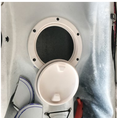
I installed a hatch just in front of my seat to put small boxes for lures and terminal tackle I use the most
